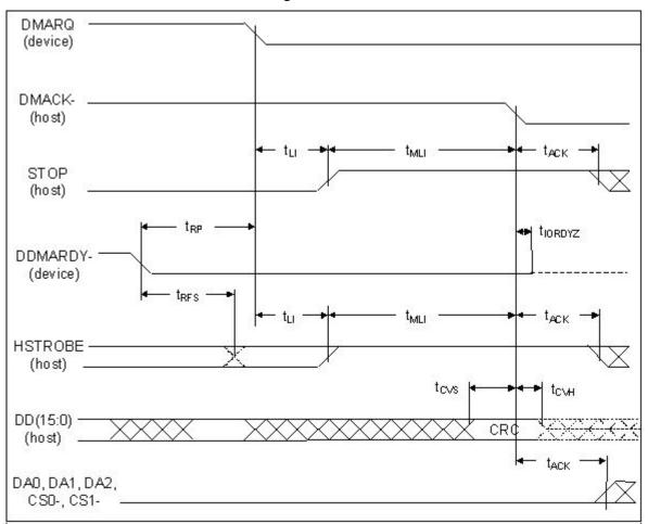
Device terminating an Ultra DMA data-out burst
