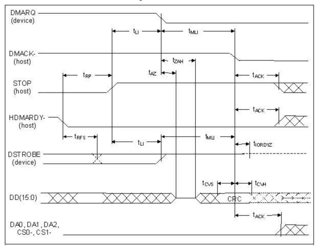
Host terminating an Ultra DMA data-in burst
