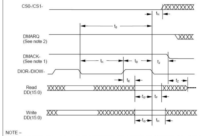
1 To terminate the transmission of a data burst, the host shall negate DMACK- within t<sub>J</sub> after a DIORor DIOW- pulse. No further DIOR- or DIOW- pulses shall be asserted for this burst.
