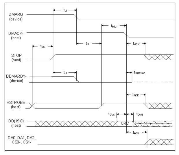
Host terminating an Ultra DMA data-out burst
